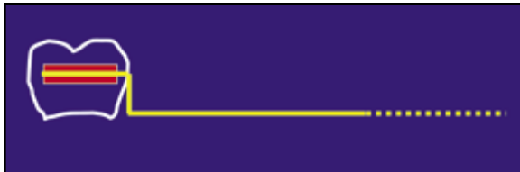
Fig. 20 In step-down arch, increased archwire length does not increase vertical deflection.
